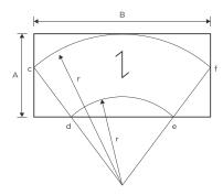
Area for invoicing AxB. Lenght of weld: cd+de+ef+fc
