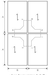
Area for invoicing 4xAxB Lenght of weld: cd+ef+gh+ij
